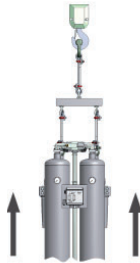
II: Installing by crane
